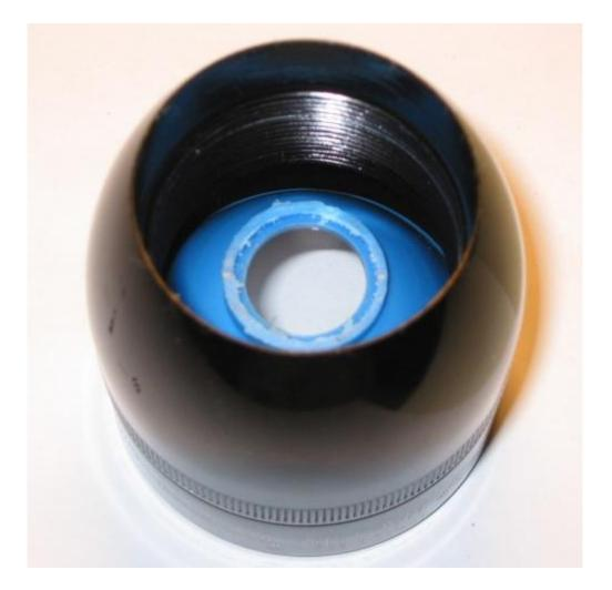
Now, fit the Hotlips into the center of the aluminium housing, pushing the resistor and the wires in. According to Hotbeam you may need to sand the interior of the aluminium housing if the Hotlips does not fit. Mine fits perfectly, provided I align it properly. You must be dead level with the tube, before it slips in with some gentle pressure.
