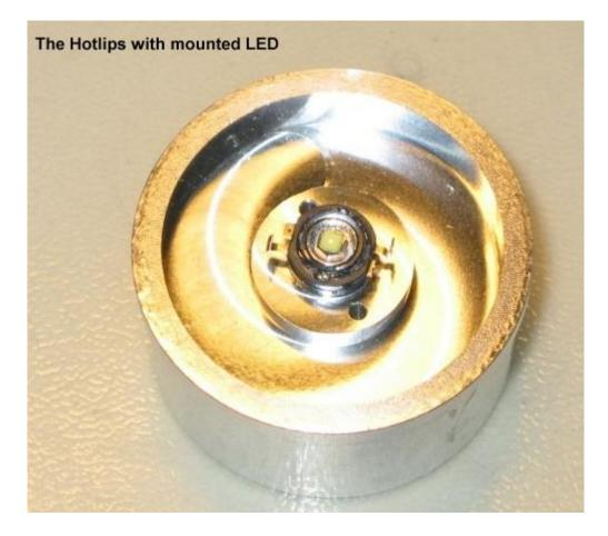
You may want to note that older OADs without a "D" in the serial number may not be able to accept the Hotlips due to differences in internal diameter. According to the link above, the D sized sinks are ~34mm, and the C-sized sinks fit newer OACs with a C in the serial number at 26.3mm. There is a conversion sleeve available for older OAC owners, please check with Hotbeam. Unfortunately, older OAD owners may be out of luck.
