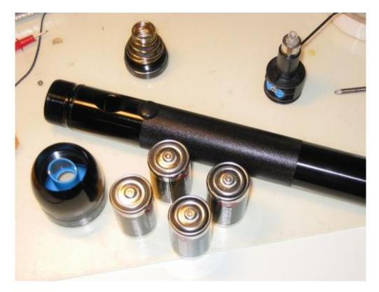
Find the copper-colored knob on the side of the bulb post of the switch assembly, stick the allen key in and unscrew the little knob. Make sure the spring-loaded bulb post does not fly out...unless you don't plan on seeing it again.
