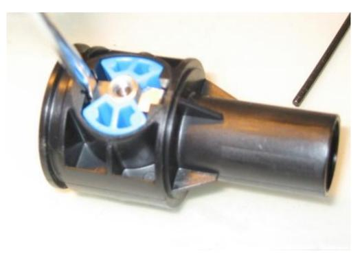
Now, saw the bulb post off. A hacksaw or a file should do it. Other unorthodox methods have been tried and can be used in a pinch, at your own risk, as always. Do not cut all the way down, you can safely leave 3-5mm as shown here :
