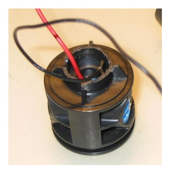
Slot the switch assembly back into the housing and use the allen key to tighten the set screw to 'fix' it back where it should be. Replace the rubber boot.
